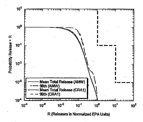
Comparison of AMW PA total releases with releases from the modified Compliance Recertification Application (CRA1). The CRA1 uses the PAVT spallings modeling instead of the spallings model used in the forthcoming (~March 26, 2004) CRA. (Source: Hansen et al. 2004, Docket A-98-49, Item II-B2-30)
