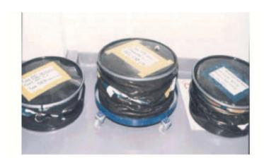
Figure 2-1. Supercompacted waste pucks as generated in the AMWTF (from Hansen et al. 2003b, Figure 2-1)
